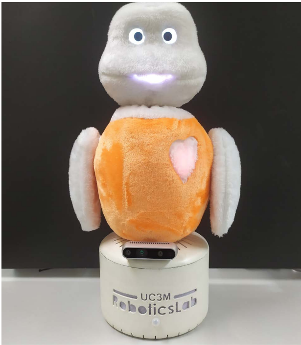
Fig. 7. Mini, a social robot developed for interacting with older adults suffering from mild cognitive impairment.
