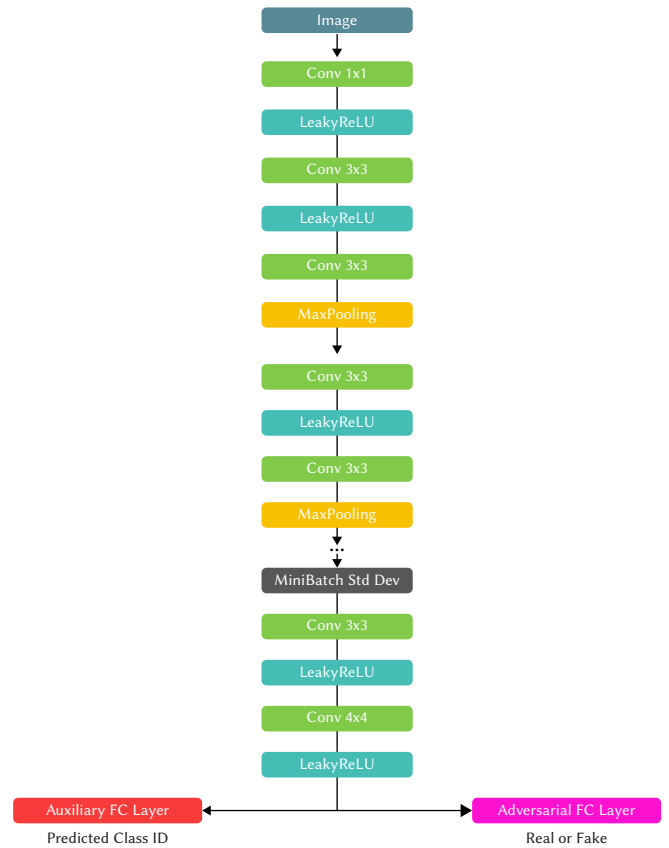
Fig. 4. Discriminator of the Style-based Generative Adversarial network with an auxiliary output block for tumor classification.
