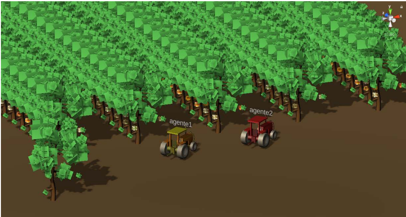
Fig. 10. Agents agente1 (yellow tractor) and agente2 (red tractor) patrolling and taking pictures of the oranges in the grove. Notice the "Tree Fruit Variant" trees with random textures of orange fruits applied at runtime, loading the images from the folder path specified in map_config.json file.
