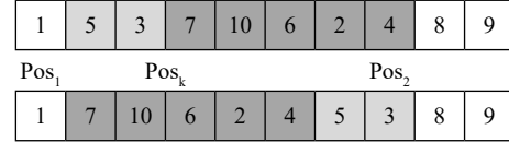
Fig. 5. Illustration of swapping mechanism.
