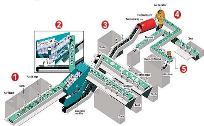
Both automated sections are in the top right. The first one consists of a red pipe which is a big magnet, its function consists of separating the metals. The yellow pipe it is a blower, it is in charge of separating the papers. The rest of the
