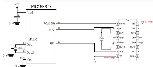
This is the scheme to make the engine work. To control the
