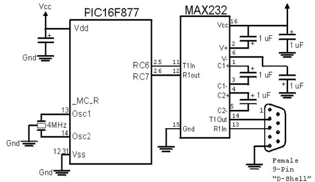
This is the scheme to obtain a correct connection with the PC. The ports of the PIC 16f877 numbers 25 and 26 are in charge of the transmission and receipt of information, in addition these ports are special since they allow the use of the USART to be able to do synchronous or asynchronous transmission of information.
